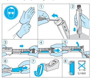
Open the handle as shown, remove the battery and dispose of it according to local environmental regulations.
